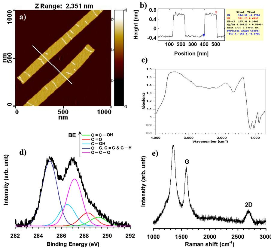
**Fig. 1.** (a) AFM image of GONRs aligned by a paint-brushing method on  $\text{Si}_3\text{N}_4/\text{Si}(1\ 0\ 0)$  substrate, (b) height profile of the ribbons marked in the AFM image indicating a thickness equivalent to the thickness of a single-layer GO (~1 nm), and (c) FTIR, (d) C(1s) core level deconvoluted XP, and (e) Raman spectra of the GONRs.
