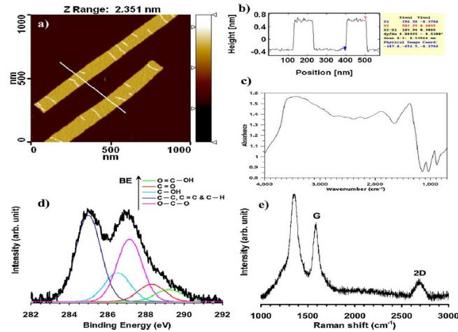
**Fig. 1.** (a) AFM image of GONRs aligned by a paint-brushing method on  $\text{Si}_3\text{N}_4/\text{Si}(100)$  substrate, (b) height profile of the ribbons marked in the AFM image indicating a thickness equivalent to the thickness of a single-layer GO ( $\sim 1$  nm), and (c) FTIR, (d) C(1s) core level of deconvoluted XP, and (e) Raman spectra of the GONRs.
