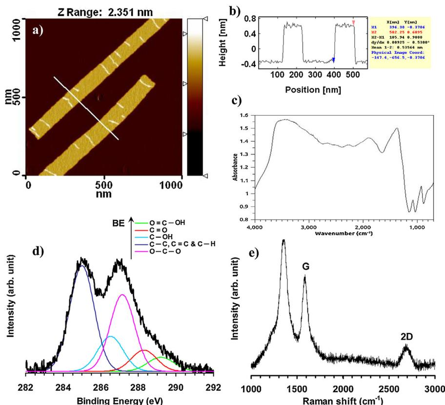
**Fig. 1.** (a) AFM image of GONRs aligned by a paint-brushing method on Si<sub>3</sub>N<sub>4</sub>/Si(1 0 0) substrate, (b) height profile of the ribbons marked in the AFM image indicating a thickness equivalent to the thickness of a single-layer GO (~1 nm), and (c) FTIR, (d) C(1s) core level of deconvoluted XP, and (e) Raman spectra of the GONRs.
