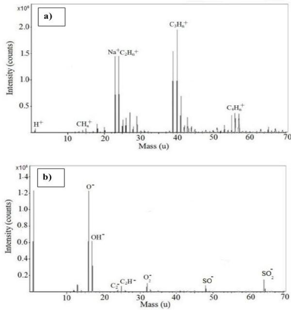
Figure 2. a) Positive and b) negative TOF-SIMS spectra of GONRs.
