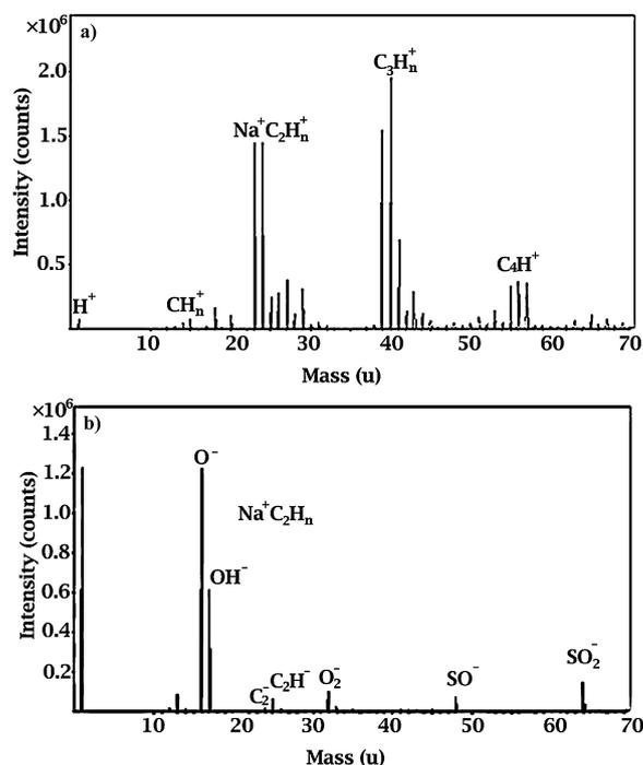
Fig. 2. (a) Positive and (b) negative TOF-SIMS spectra of GONRs.
