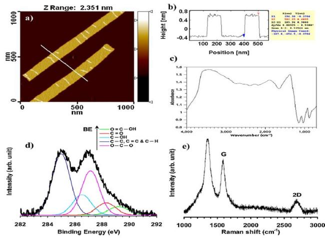
Fig. 1. (a) AFM image of GONRs aligned by a paint-brushing method on  $\text{Si}_3\text{N}_4/\text{Si}(100)$  substrate, (b) height profile of the ribbons marked in the AFM image indicating a thickness equivalent to the thickness of a single-layer GO (~1 nm), and (c) FTIR, (d) C(1s) core level of deconvoluted XP, and (e) Raman spectra of the GONRs.
